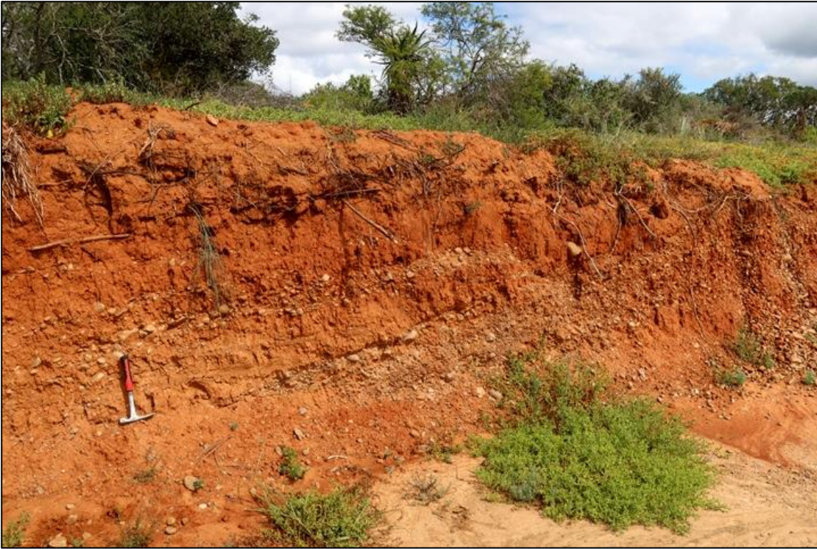
Figure 8: Vertical section through thick sandy alluvial deposits of the valley floor with cross-bedded gravel bars exposed by recent excavations c. 600 m SE of the proposed new dam wall site (hammer = 30 cm).
