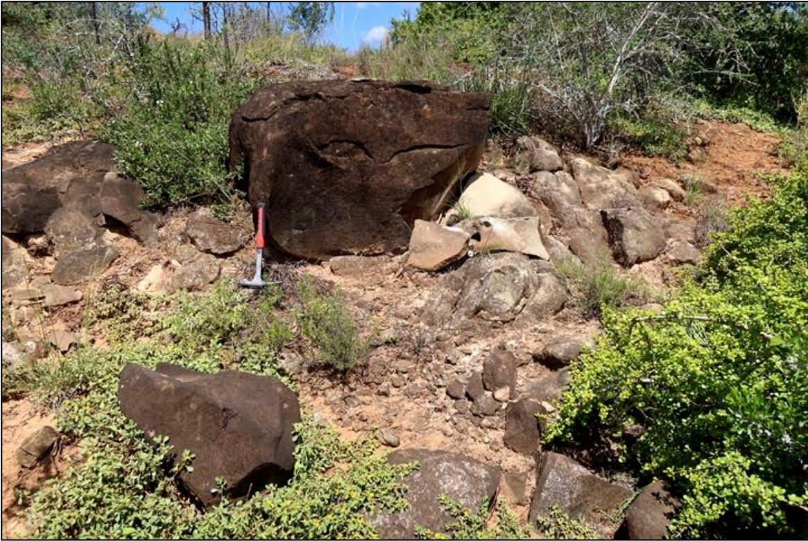
Figure 6: Low scarp or krans of jointed, grey-green Sundays River Formation sandstone towards the SW edge of the dam basin project area showing typical dark brown weathering patina (hammer = 30 cm).
